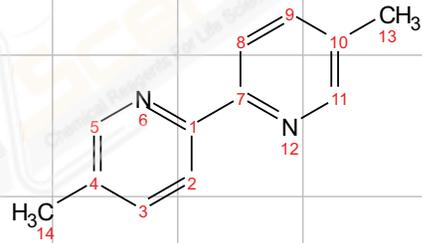
$^1\text{H NMR}$  (400 MHz, Chloroform-*d*)  $\delta$  8.48 (dt,  $J = 2.3, 0.8$  Hz, 2H), 8.23 (dd,  $J = 8.1, 0.8$  Hz, 2H), 7.60 (ddd,  $J = 8.0, 2.3, 0.8$  Hz, 2H), 2.37 (s, 6H).
